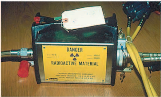
A radioactive source shield with warnings . . .
