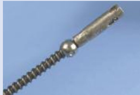
PH33. Photo of a vary dangerous ionizing source from a radiography machine
