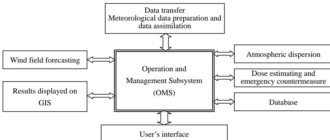
Data transfer and pre-processor module is in charge of interface between the system and outside, such as acquiring meteorological data from SQL server database in local area network, carrying out preparation of all model-input parameters and releasing the results to the server of local area network.
