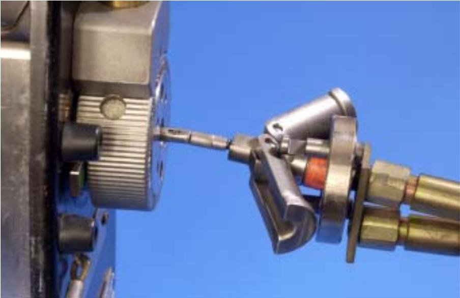
*FIG. 5. Drive cable connected to the source pigtail. The two parts of the cylindrical metal collar are in the open position.*
