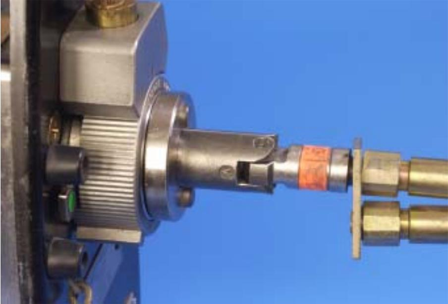
*FIG. 8. The lugs are fully engaged and the locking ring is rotated to hold the drive cable captive.*
