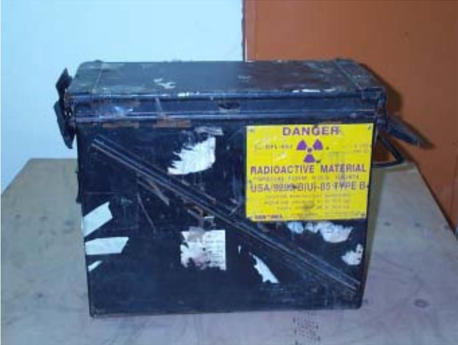
*FIG. 9. Overpack for the source container.*
