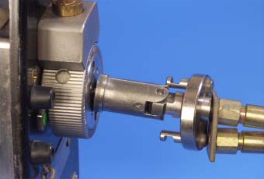
*FIG. 6. The two parts of the cylindrical metal collar are closed over the connector (to the right of the connector is a disc with keyed metal lugs).*
