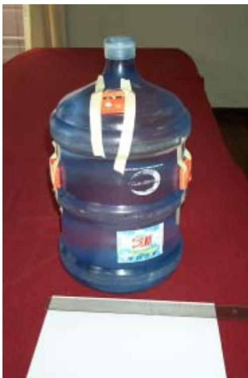
*FIG. 19. Water bottle as used in lieu of human phantoms for the reconstruction of the dose.*
