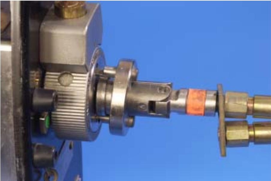
*FIG. 7. The metal lugs enter the locking ring.*
