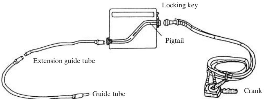
FIG. 3. Schematic view of the remote exposure container and ancillary equipment involved in the accident in Cochabamba.
