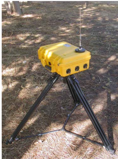
Figure 1: Deployed Radiation Monitoring Station
