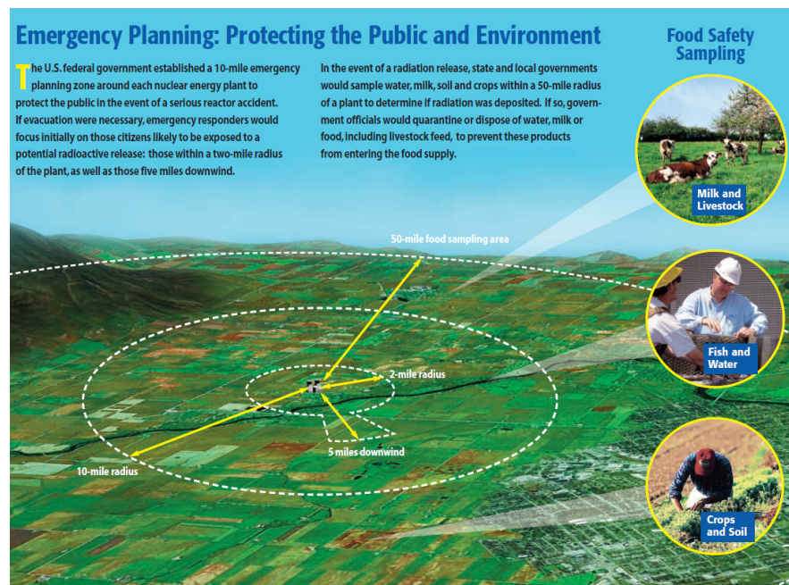
Figure 2. U.S. Emergency Planning Zones for a Nuclear Power Plant
